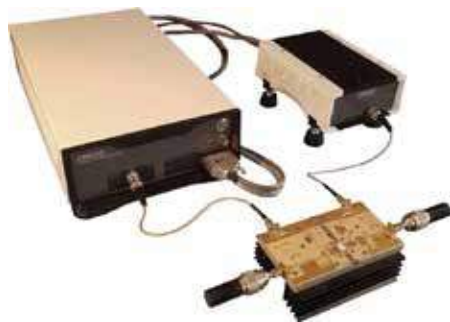
AM3100 used for pulsed bias of Power Amplifiers
