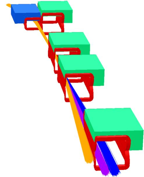
H<sup>-</sup>, H and proton beams through ISIS injection magnets
